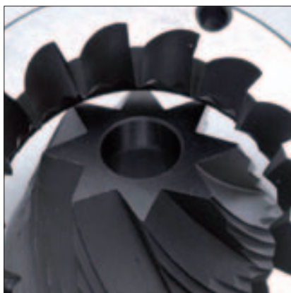
Macine coniche Conical burrs
